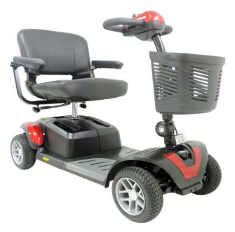
The AGIS M9 Mid Size Luxury Mobility Scooter comes with all wheels suspension that deliver a smooth and comfortable ride on all terrain, front and back Ultra Bright LED light for safety and larger floor board of 450mm wide to give ample foot rest space and one wide angle Rear Mirror.
