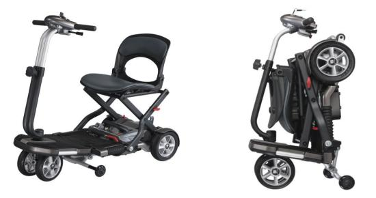
Built in Taiwan with durable aluminum chassis and tiller with a total weight less than 27KG. Folded scooter easily rolls along like a travelling suitcase. A scooter that you can bring along for holiday oversea. Compliant with IATA Air Travel requirement.
